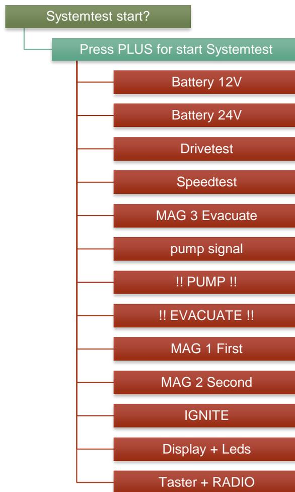
This menu item is used to start different internal system tests. They should only be made after being instructed by qualified personnel.
